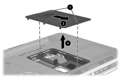
Removing the Memory Expansion/Mini PCI Compartment Cover
